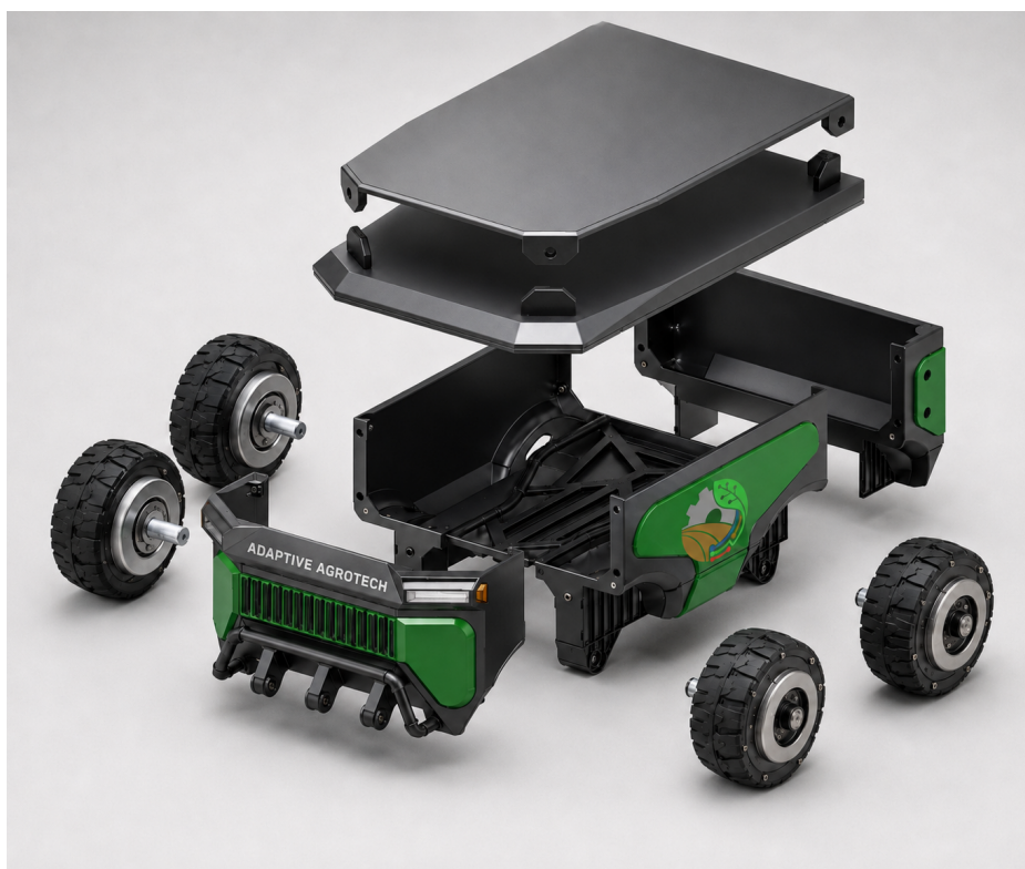
Figure 7. Exploded concept visualization showing top covers, body structure and four hub-wheel assemblies. The separated parts illustrate modularity; the image is not a service disassembly sequence or an as-built electrical drawing.
